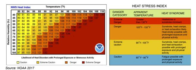
Figure 7. Heat Index Chart and Heat Stress Levels
