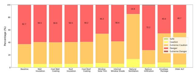
Figure 16. Percentage of Hours at each Heat Index Level of the Baseline and Mitigated Assisted Living Facilities with Passive Measures During the 2015 Heatwave
