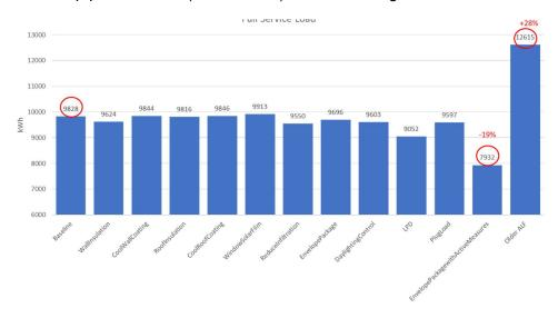
Figure 19. Back-up Power Capacity to Provide Full-service Loads for the 2021 Cold Snap
