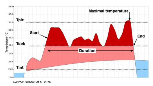
Figure 4. Identification of an Extreme Heat Event using Daily Mean Temperature as an Indicator
