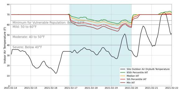
Figure 14. Hourly Indoor Air Temperature Distribution and Outdoor Air Dry-Bulb Temperature of Baseline Assisted Living Facility Model in 2021 Snowstorm
