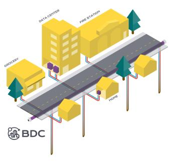
Illustration of a geothermal network along a street. Water circulates through boreholes and a shared loop of pipe to deliver temperature to ground source heat pumps in connected buildings.
